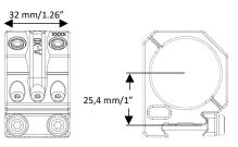
The rings are machined from billet 7000 series aluminum and all aluminum parts are hardcoat anodized. The Torx 20 ring and clamping screws are zinc-nickel coated for corrosion resistance and come pre-waxed from the factory to ensure proper torque values.
